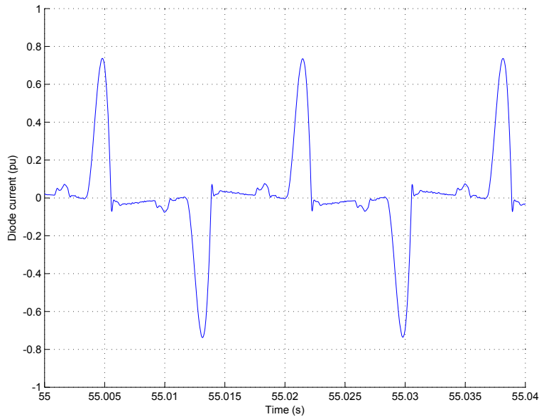
Figure 5.4. Rectifier current under 2% unbalanced grid voltage.
